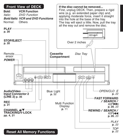
Returns to factory setting. Use if relocating DECK, or if Initial etup needs to be redone.
